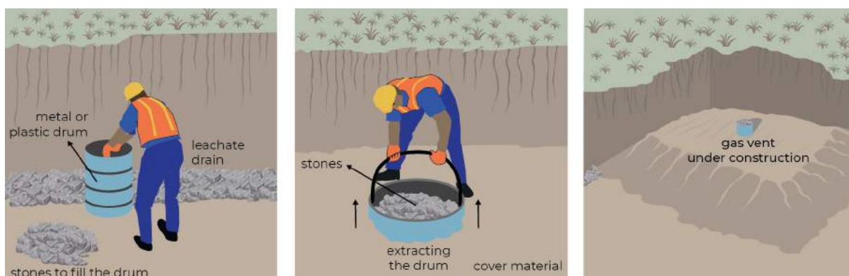
Figure 23: Gas vent construction
