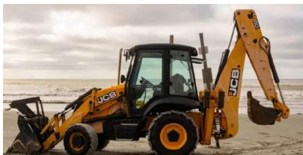
Figure 14: Tractor with front-end loader and rear digging bucket (photo credit: Farming Base, n.d.)
