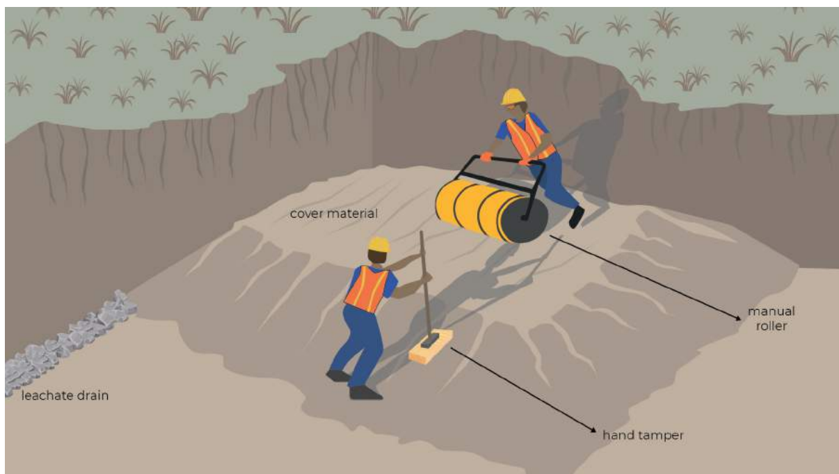
Figure 11: Final compaction and closure of the cell
