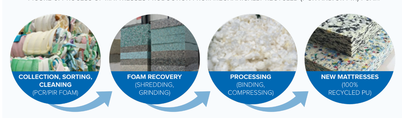
FIGURE 6. PROCESS OF MATTRESSES PRODUCTION FROM MECHANICALLY RECYCLED (PCR AND/OR PIR) FOAM
