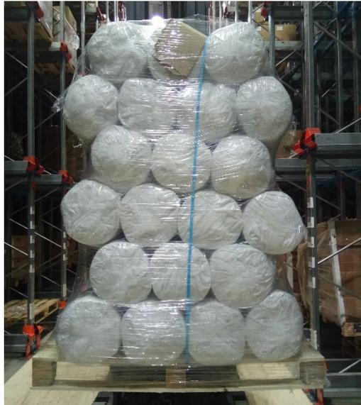
Two or more plastics hoops should be placed to protect the edges not to deform the layer.
