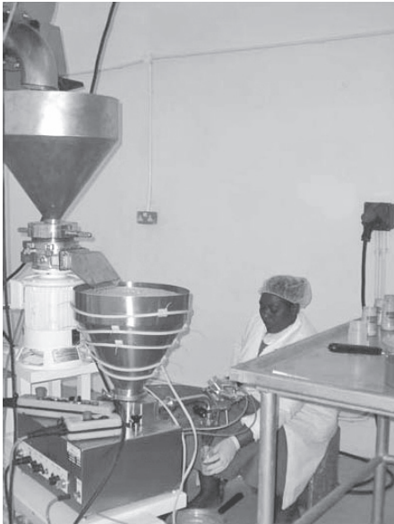
FIG. 3. Single mixing and packaging unit for large-scale production of ready-to-use therapeutic food (RUTF)
