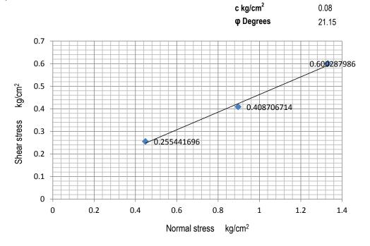
Remarks: The sample was sieved through sieve No. 8 prior to conducting this test.
