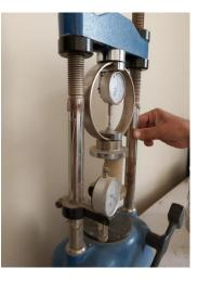
strength for those soils that possess sufficient cohesion to permit testing in the unconfined state.
