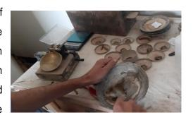
range of water contents over which a soil behaves plastically is termed the Plastic Index and corresponds to the numerical difference between the liquid and plastic limit (ie, W<sub>r</sub>W<sub>P</sub>).
