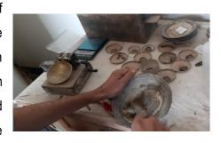
range of water contents over which a soil behaves plastically is termed the Plastic Index and corresponds to the numerical difference between the liquid and plastic limit (ie, W<sub>r</sub>W<sub>P</sub>).
