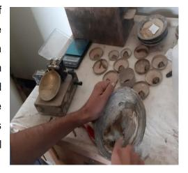
The liquid limit (LL) is arbitrarily known as the water content, in percent, at which a pat of soil in a standard cup and cut by a groove of standard dimensions will flow together at the base of the groove for a distance of 13 mm (1/2 in.) when subjected to 25 shocks from the cup being dropped 10 mm in a standard liquid limit apparatus operated at a rate of two shocks per second. The typical cassagrande's apparatus was used in determination of Liquid Limit.
