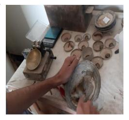
The liquid limit (LL) is arbitrarily known as the water content, in percent, at which a pat of soil in a standard cup and cut by a groove of standard dimensions will flow together at the base of the groove for a distance of 13 mm (1/2 in.) when subjected to 25 shocks from the cup being dropped 10 mm in a standard liquid limit apparatus operated at a rate of two shocks per second. The typical cassagrande's apparatus was used in determination of Liquid Limit.
