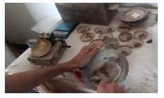
fine grained soils. They are expressed in percentage water content. The range of water contents over which a soil behaves plastically is termed the Plastic Index and corresponds to the numerical difference between the liquid and plastic limit (ie, W<sub>r</sub>W<sub>P</sub>).
