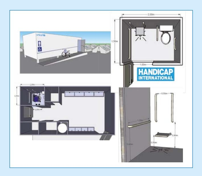
Handicap International provided guidance for the design of WASH blocks for Zaatari Camp in Jordan in 2012. The images above were part of a guidance note developed on accessible WASH blocks<sup>10</sup>.
